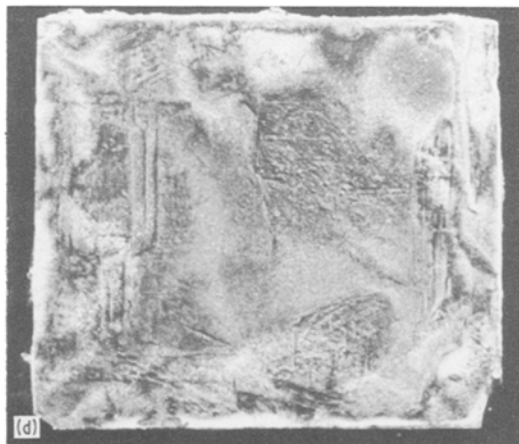
Figure 3 Natural diamond specimen GH2, surface designated “b”. Photographs printed left-to-right to assist comparison with Fig. 1. (a) Cathodoluminescence topograph; (b) Magnetic tape developer pattern after corona charging as in Fig. 1b, specimen mounted on silicone rubber compound; (c) Pb_3O_4 pattern obtained in a similar way to that shown in Fig. 1c; (d) MgO pattern obtained after triboelectric charging of specimen.
